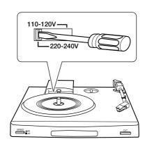
Move switch lever to match your line voltage with a small screwdriver or other pointed tool.
